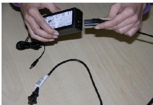
Figure 3 Assemble power cord to low voltage transformer
